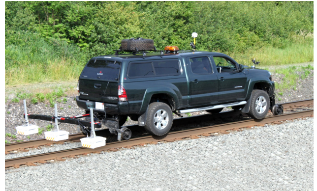
Road-rail vehicle equipped with SRS
